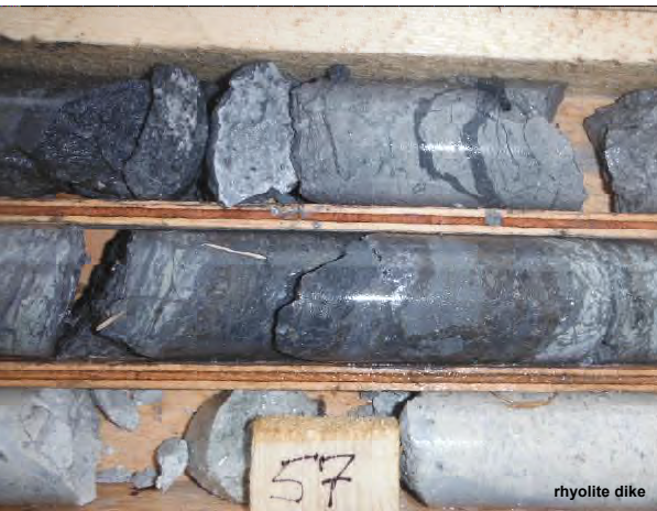
Hole G18-01, quartz-sulfide vein at 56.2m 0.5m @ 863 g/t Ag, 1.4 g/t Au, 6.75% Pb and 9.6% Zn
