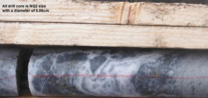
Hole G18-01, quartz-sulfide vein at 56.2m 0.5m @ 863 g/t Ag, 1.4 g/t Au, 6.75% Pb and 9.6% Zn
